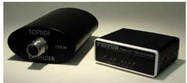
Left: Remote Ethernet Extender (in waterproof housing) Right: Local Ethernet Extender
