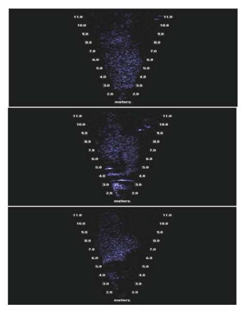
Scale tool. While there is a decrease in resolution with increasing distance from the transducer, measurements taken at 6 m did not differ by more than 2 cm across the 1- to 12-m range.
