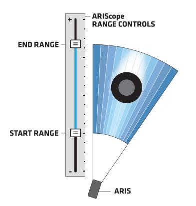
The width of the acoustic wedge is a fan of narrow slices. Each slice from a beam of ARIS produces a thin strip of the image aligned with range which is placed appropriately with neighbors in cross range to produce the entire image.
